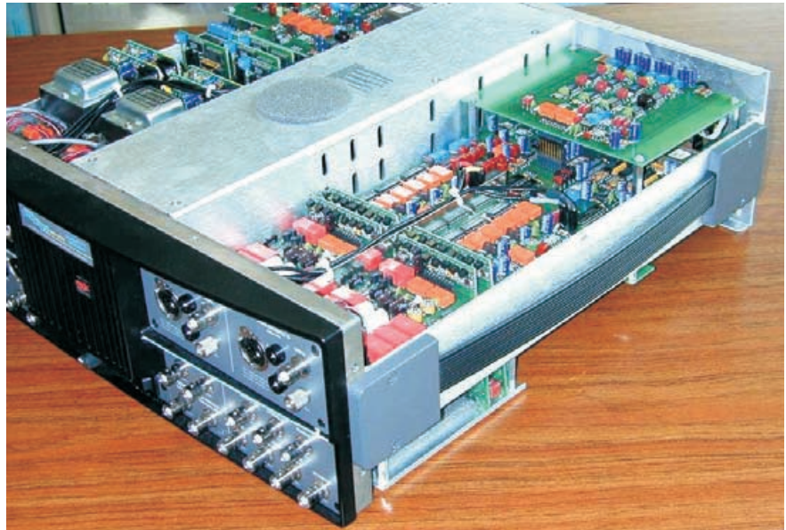
Figure 3-1. System Two Cascade with covers removed (shown with filter installed). System Two is mechanically similar.
